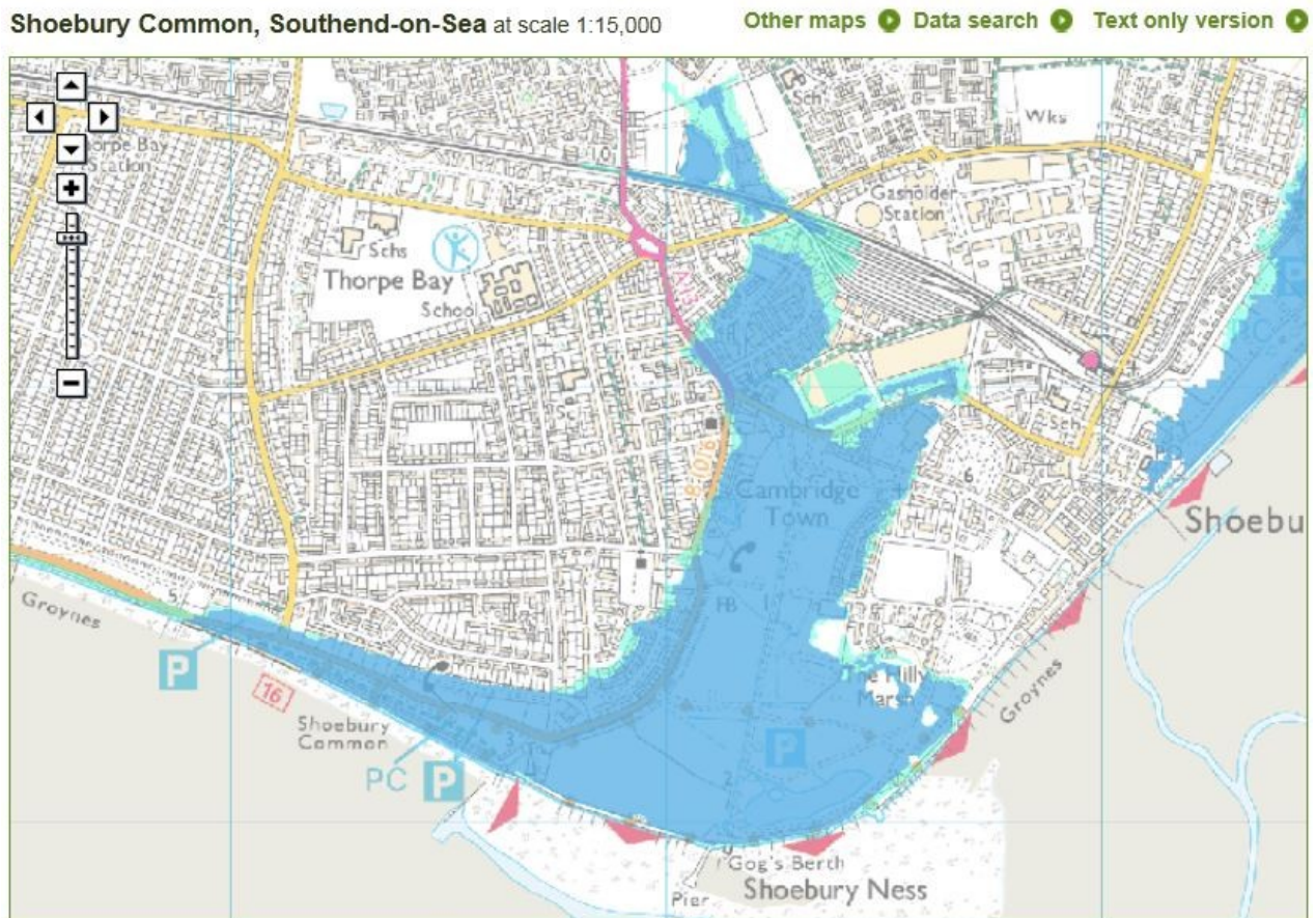
Figure 2.4: Shoebury Common Flood Map showing 1 in 200 year (dark blue) and 1 in 1000 year (light blue) return period coastal flood event.
