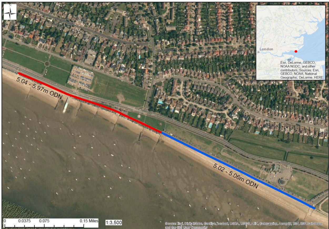
Figure 2.1: Variation in seawall elevation along the Shoebury Common frontage. Levels at the west section (red) vary between 5.04 and 5.88m ODN. Levels at the east section (blue) vary between 5.02 – 5.06m ODN.
